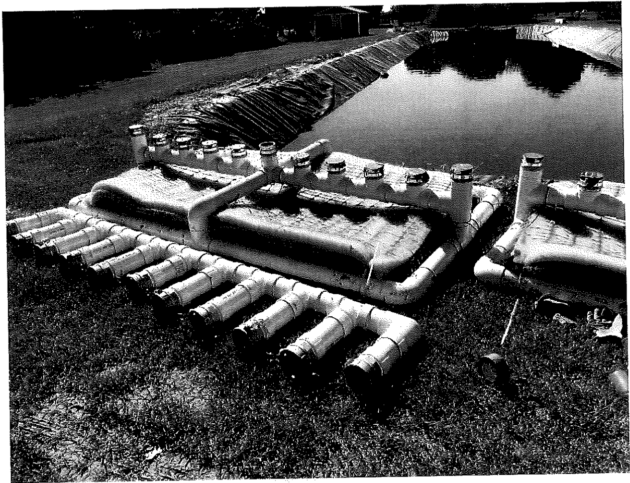
Figure 11. Floating wetland breakwater frame used for the prototype system (upside-down). Photo by Maxwell O'Brien.
