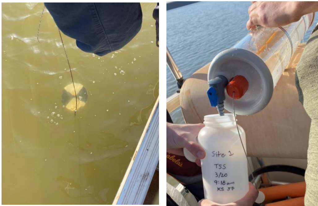
Figure 9: Secchi Dish Depth Measurement; Figure 10: Van Dorn Sampler Collection of Water Sample and Sample Labeling
